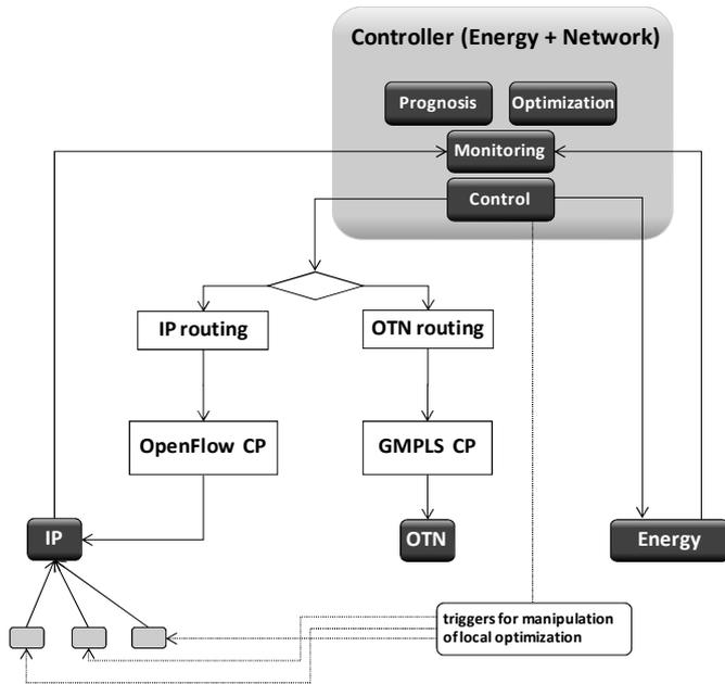
Fig. 3: Control architecture of the DESI solution: consistent treatment of telco network and energy degrees of freedom.
