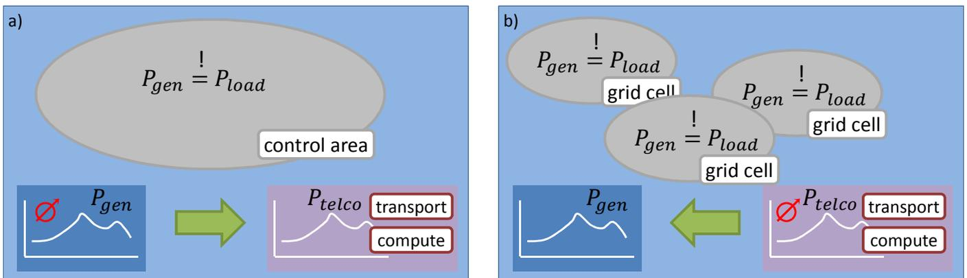
Fig. 1: Principal changes in the energy provisioning of the telco network; from traditional system (a) to the *Smart Energy* system (b).
